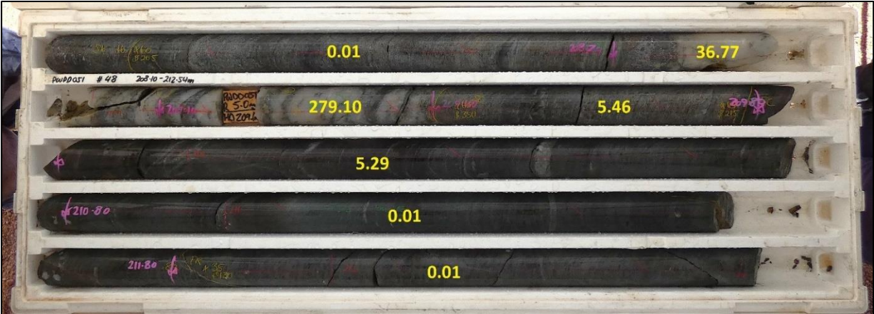
Figure 7: Diamond drill core from hole PWDD051 showing the Penny West laminated quartz vein with an intercept of 2.0m at 51.0g/t Au from 208.8m including 0.3g/t at 279g/t Au from 209.1m.
